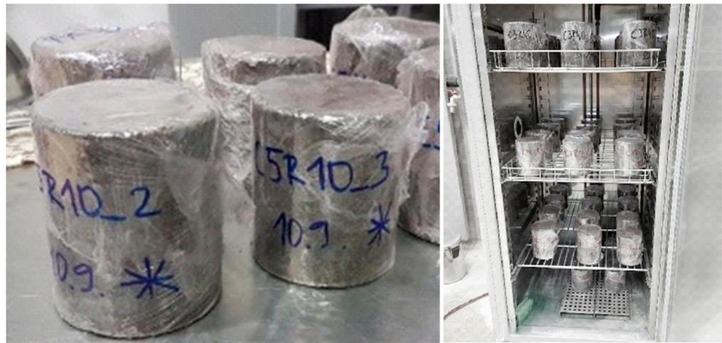
**Figure 3.** Samples for compressive strength and RTF determination.
