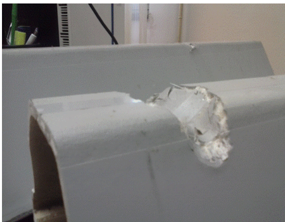
Figure 4. Photograph of beam deformation
