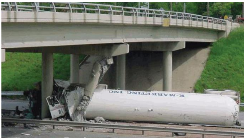
Figure 1 Impact between vehicle and column (U.S. highway) [8]
