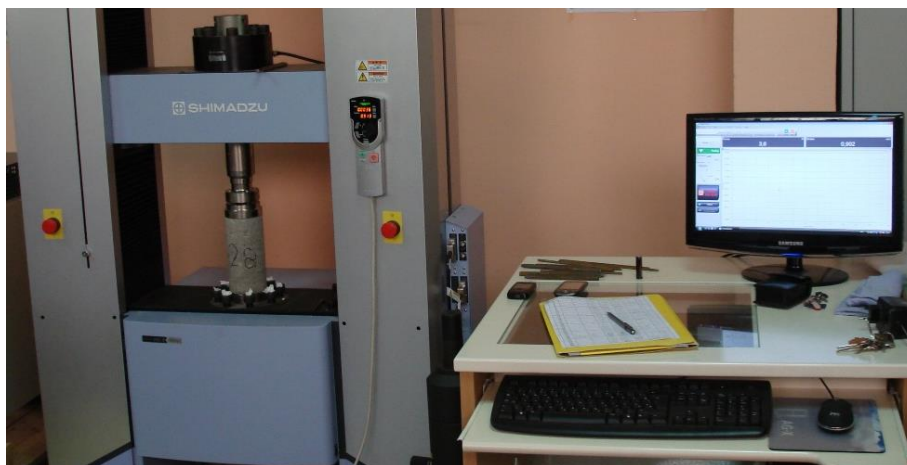
Figure 3 Equipment used to test compressive strength
