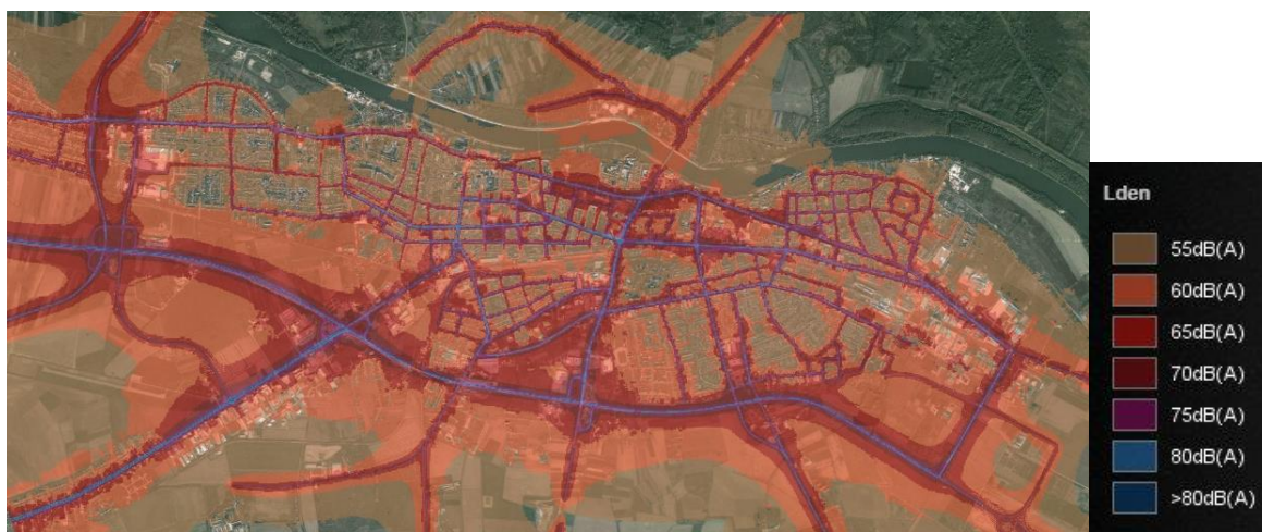
Figure 2 Daylong ( L_{den} ) noise levels from road traffic
