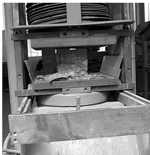
Figure 3 Compression failure of the brick Slika 3. Tlačni slom opeke
