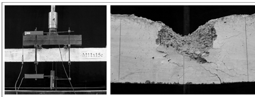
Figure 8 Failure of an over-reinforced concrete beam [7] Slika 8 Slom prearmirane betonske grede [7]
