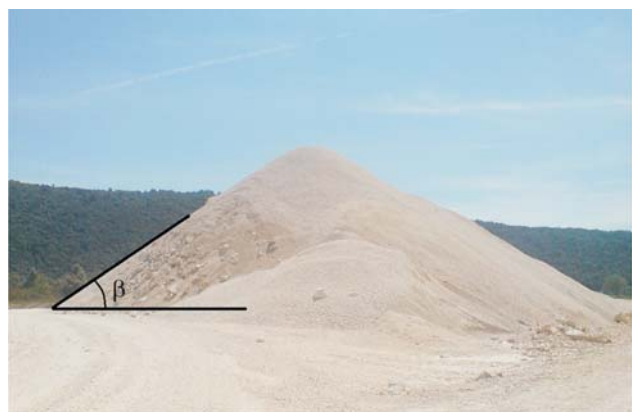
Figure 2 Formation of cone of soil with natural repose angle \beta for non-cohesive soil
