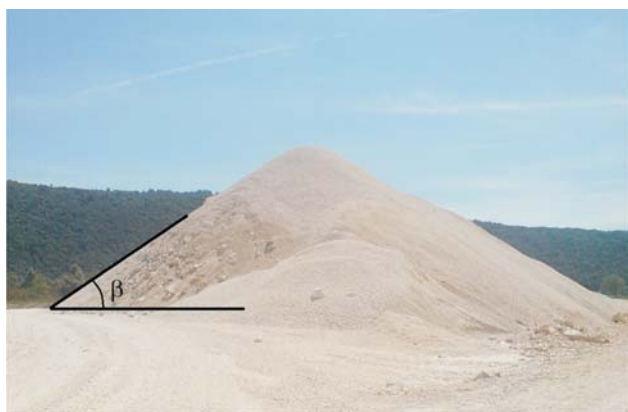
Figure 2 Formation of cone of soil with natural repose angle \beta for non-cohesive soil
