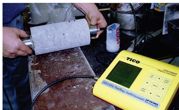
Figure 2 Measurement of ultrasound pulse velocity
