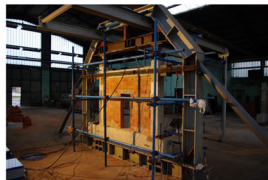
Fig. 2 Infilled frames tested by (Penava 2012)
