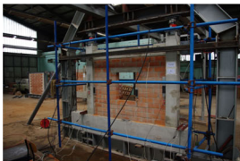
Fig. 2 Infilled frames tested by (Penava 2012)
