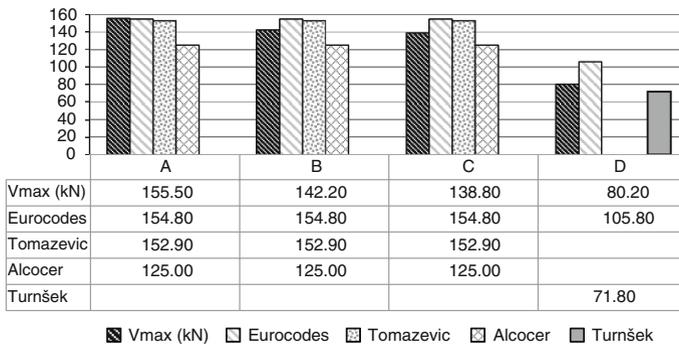
**Fig. 17** Calculated and experimental lateral shear resistance of the tested specimens
