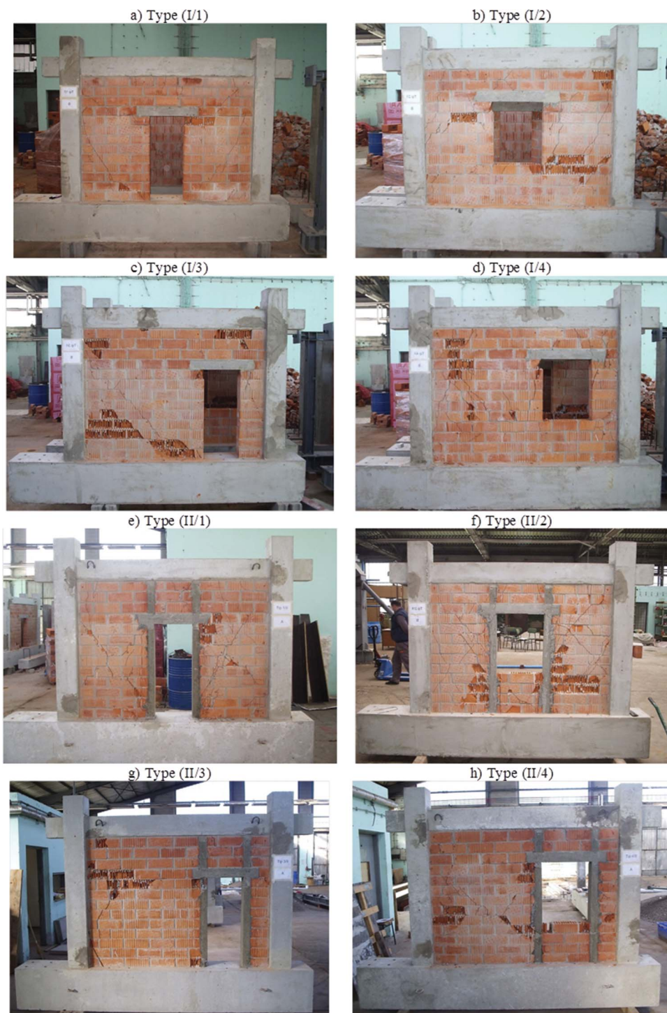
FIGURE 5 Specimens after the test (color figure available online).
