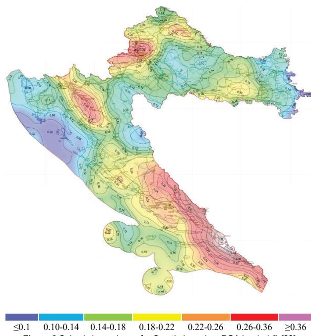
Figure 2 Seismic hazard map for Croatia based on PGA in g(m/s<sup>2</sup>) [23]
