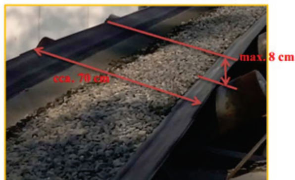
Figure 3 Dimensions and appearance of the incline conveyor belt
