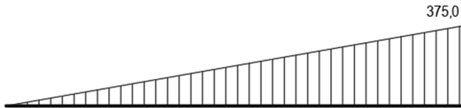
Dijagram poprečnih sila,  $V_{z,Ed}$  [kN]
