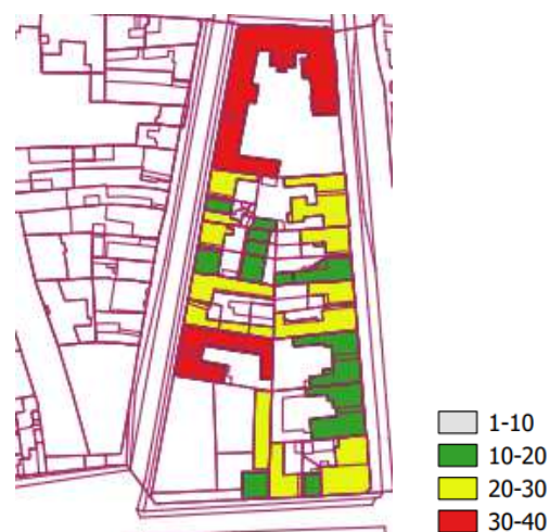
Figure 4. The seismic priority index (SPI) obtained for earthquake intensity VII
