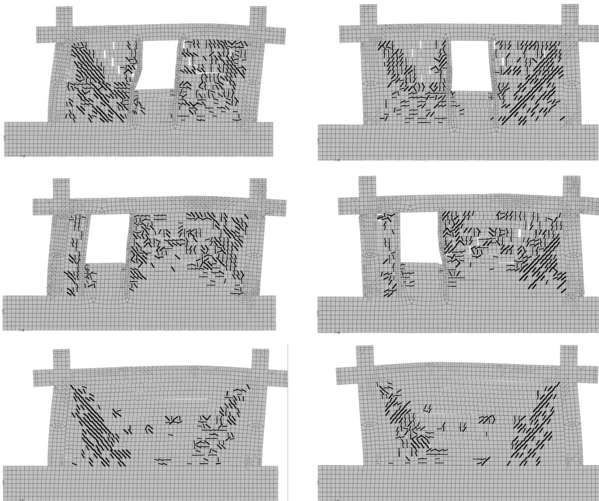
Slika 6.13. Oštećenost pred slom za IDR=1,0 % modela tip (V/1), tip (V/2) i tip (V/3)
