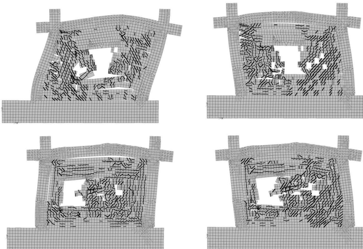
**Slika 6.5.** Oštećenost pred slom za IDR=1,0 % modela tip (IV/5) gore i tip (IV/6) dolje
