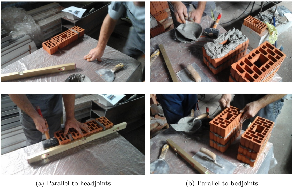
Figure 4.3: Preparation of masonry triplets tests (Penava, 2012)
