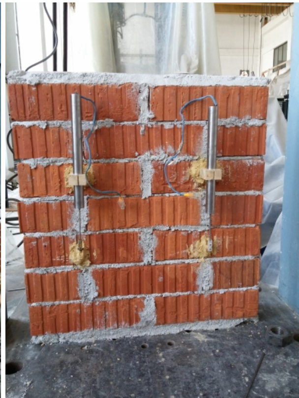
(c) LVDT placement
