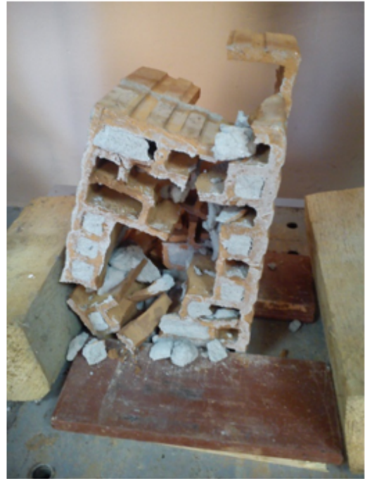
Figure 4.4: Tensional failure parallel to bedjoints (Penava, 2012)
