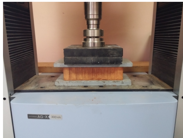
(b) In direction of voids
