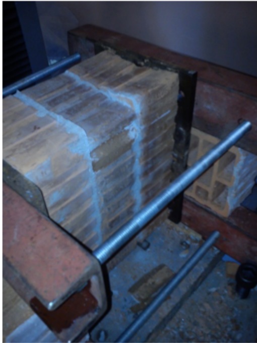
Figure 4.4: Tensional failure parallel to bedjoints (Penava, 2012)
