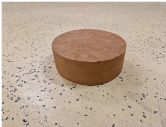
Figure 5. Experimental specimen for the Fox 200
