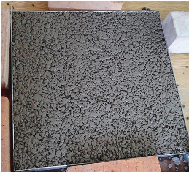
Figure 3. Pervious concrete slab for sound spectral analyses.
