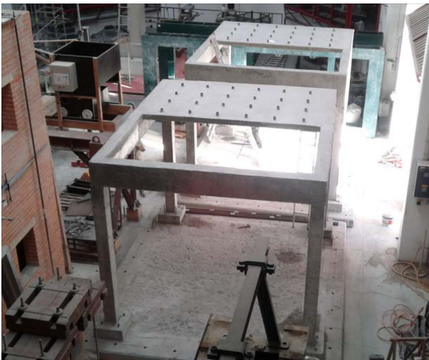
Figure 1. General view of the frame after formwork removal [16].
