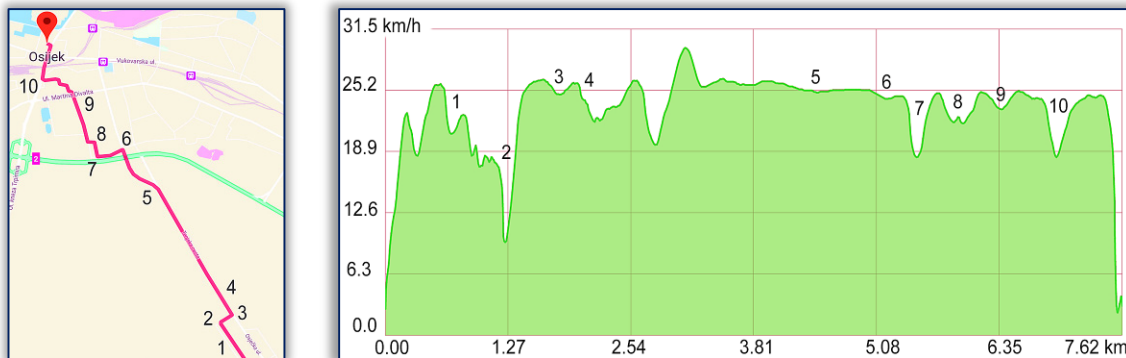
Figure 2. The basic daily route of PEDELEC and the driving dynamics of the daily route, source [2]
