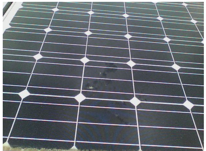
Figure 8. The surface of the panel covered with bird droppings
