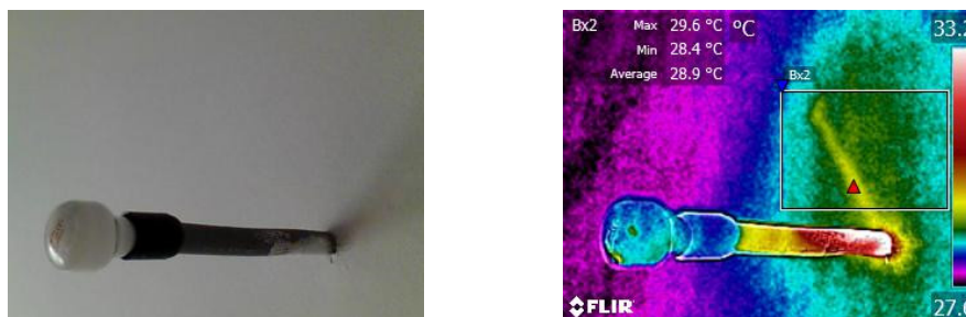
Figure 12. Finding a power supply cable with active thermography.
