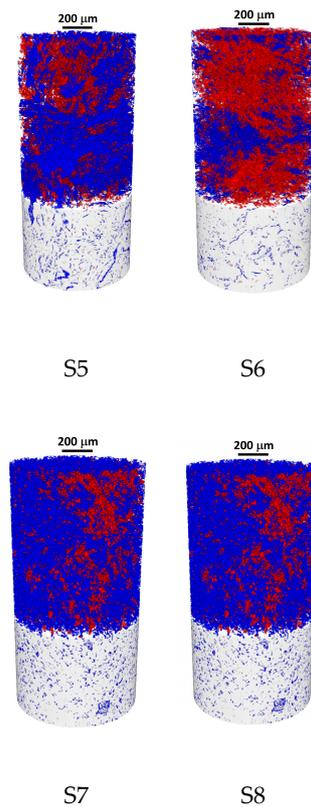
**Figure 3.** Characteristic micro-CT images of brick samples illustrating the quantitative differences reported in Table 3 (closed pores are marked in red, open pores in blue and the matrix is colored grey).
