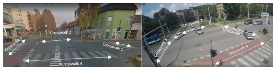
Figure 3. Intersection A (left)—crosswalks 1 and 3 on collector road and crosswalks 2 and 4 on primary road; Intersection B (right)—crosswalks 1 and 3 on primary road and crosswalks 2 and 4 on collector road.
