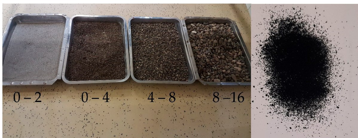
Figure 1. Natural aggregate and waste rubber used.
