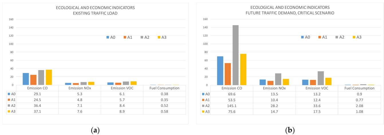
Figure 6. Comparison of gas emissions and fuel consumption for the existing traffic load (a) and for future traffic demand (b).
