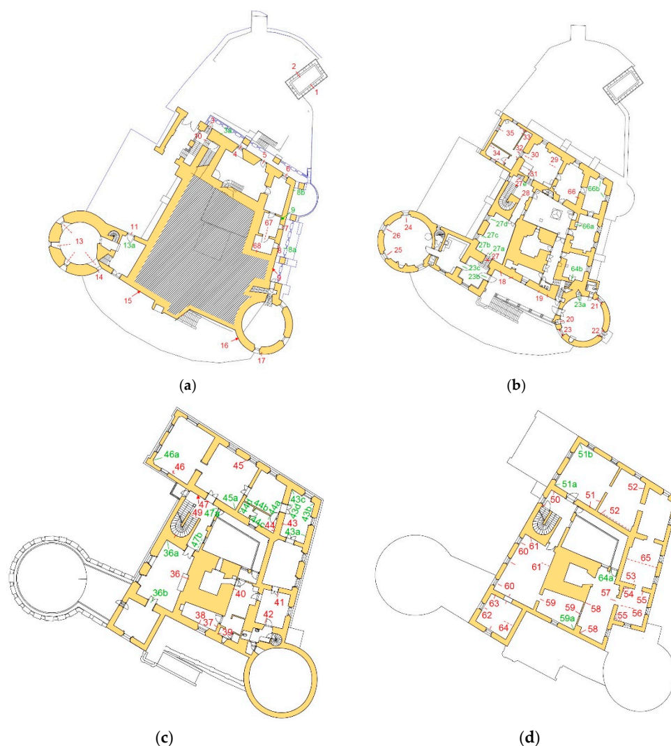
Figure 10. Map of crack positions observed during the in situ visual inspection: (a) Basement; (b) Ground floor; (c) First floor; (d) Second floor (note: red colored marks designate the damage after the Zagreb M5.5 2020 earthquake and green colored marks designate damage after the Petrinja M6.2 2020 earthquake).
