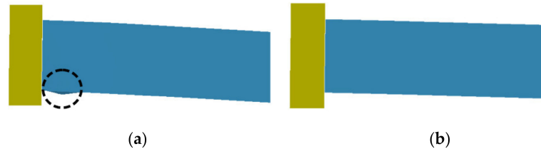
Figure 19. Failure mode of CFDST column with: (a) normal strength concrete and (b) UHPC [21]. Copyright permission obtained from authors.
