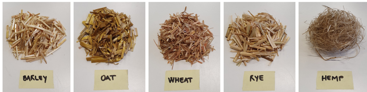
Figure 5. Cereal straw and hemp fibers used for mixtures M7–M11.
