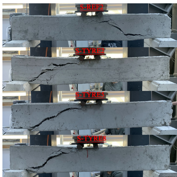
Figure 10. Damage views of the reference sample and samples with 20 cm transverse reinforcement spacing and RSWT ratios of 1%, 2% and 3%.
