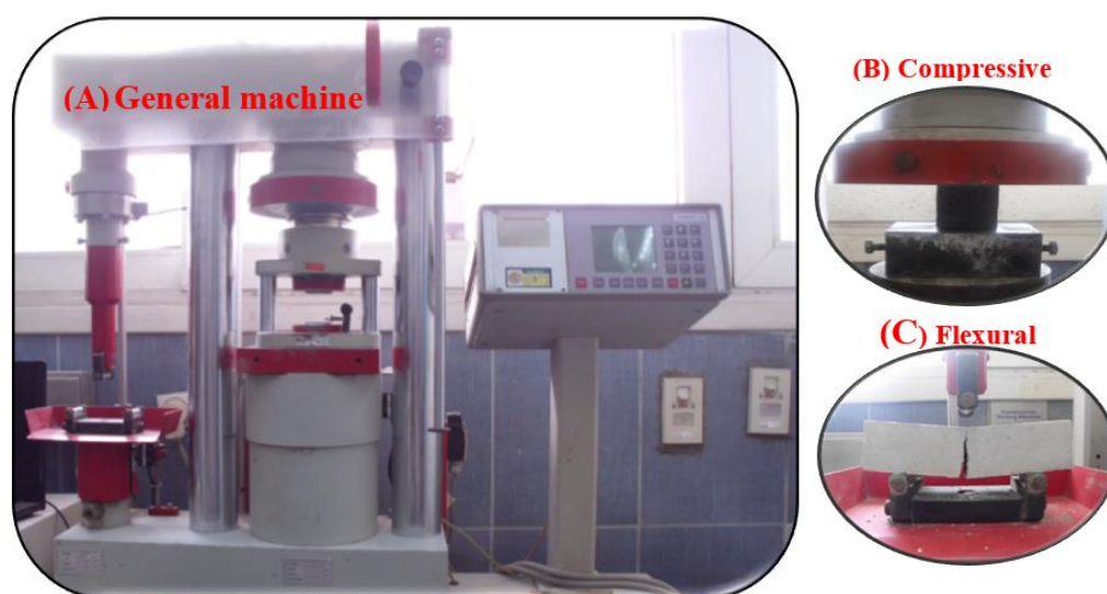
Figure 4. View of testing: (A) machine, (B) compressive strength, and (C) flexural strength.
