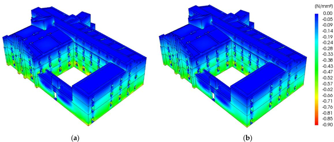
**Figure 12.** Vertical stresses due to the gravity load combinations applied following the code requirements: (a) Load combination LC<sub>1</sub>; (b) Load combination LC<sub>2</sub>.
