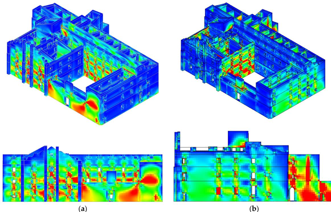
**Figure 15.** In-plane shear stresses resulting from the seismic load combinations: (a) Load combination LC<sub>3</sub>; (b) Load combination LC<sub>4</sub>.
