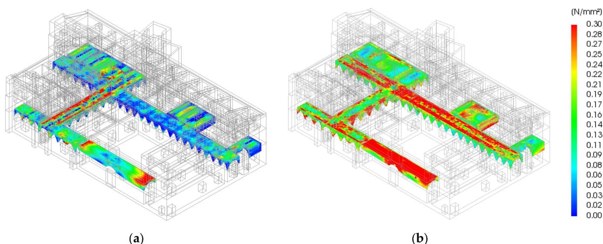
**Figure 14.** Tensile stresses in the vaults resulting from the seismic load combinations: (a) Load combination LC<sub>3</sub>; (b) Load combination LC<sub>4</sub>.
