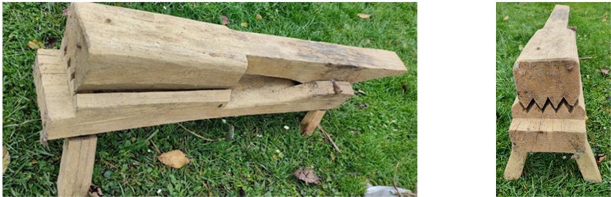
**Figure 4.** Wooden stand for fiber extraction.
