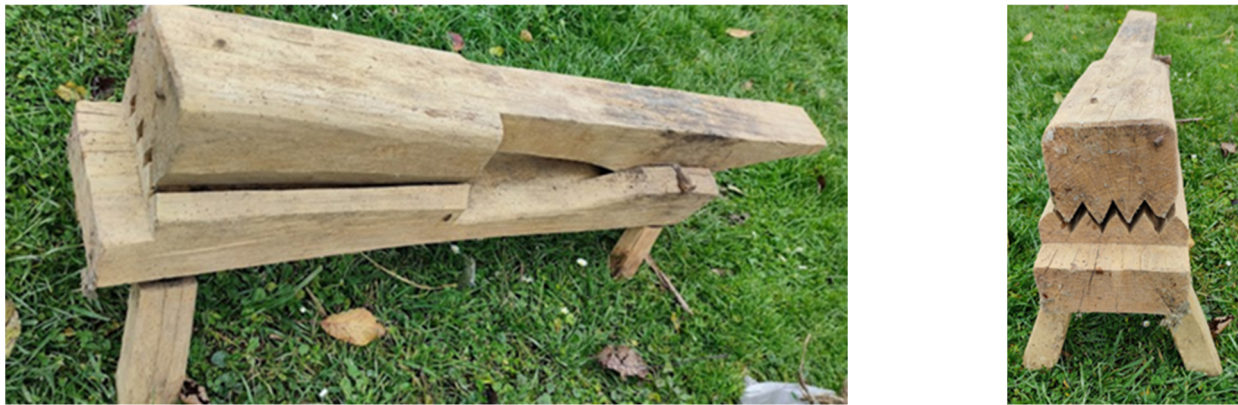
Figure 4. Wooden stand for fiber extraction.
