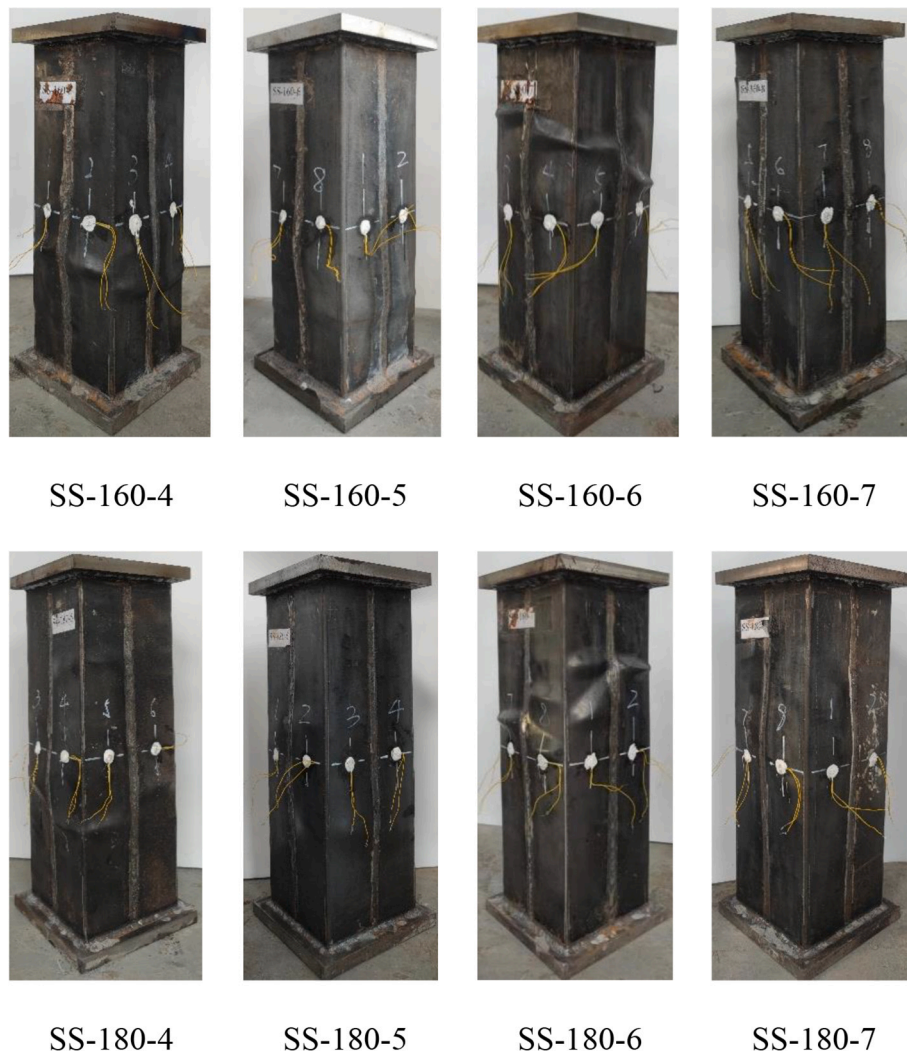
Fig. 10. Failure modes of test CFDSST columns with varying values of t_o or B .
