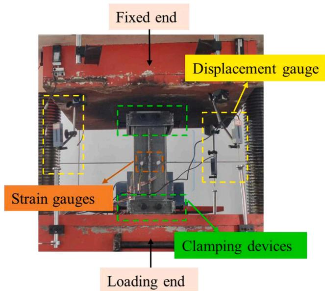
Fig. 8. Experimental test setup and clamping device.
