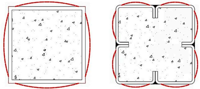
Fig. 2. Buckling modes of steel and composite sections.
