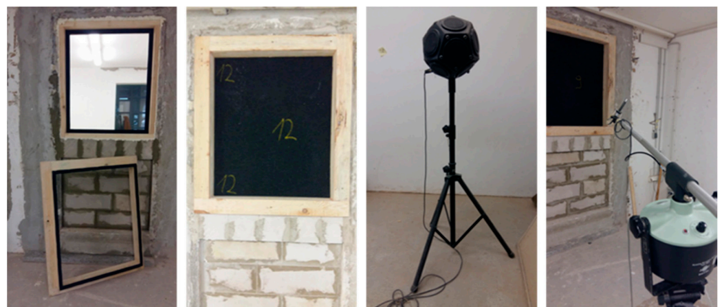
Figure 7. Airborne sound insulation index test setup.
