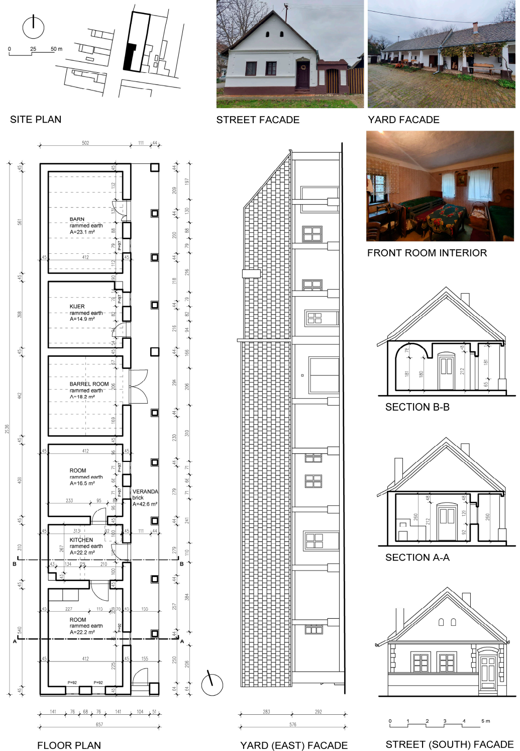
Figure 3. Floor plan, section, façade, and interior and exterior photographs of the house in Bijelo Brdo with the gable facing the street. Author’s photos and drawings.
