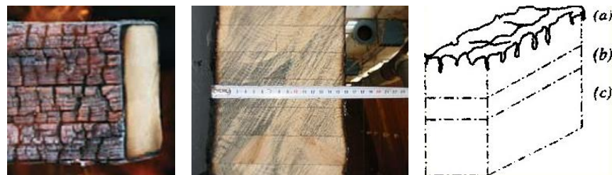
Figure 1. Degradation of timber at high temperatures (a) a layer of timber charring, (b) a layer of pyrolysis, (c) unchanged timber.
