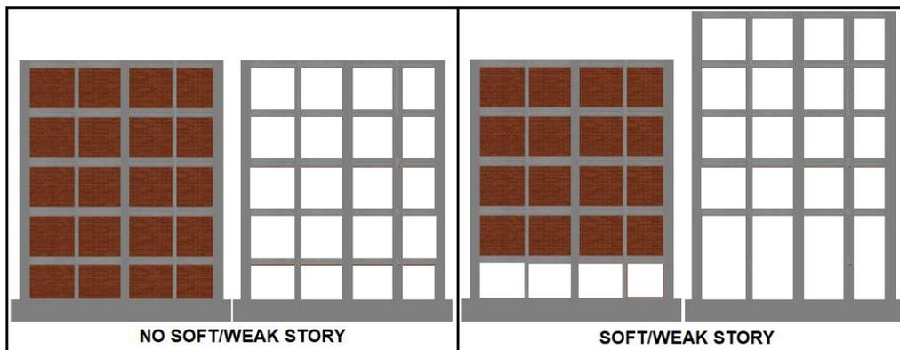
Figure 4. Detection of soft/weak storey in RC structures.
