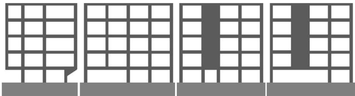
Figure 5. Vertical irregularities in RC structures.
