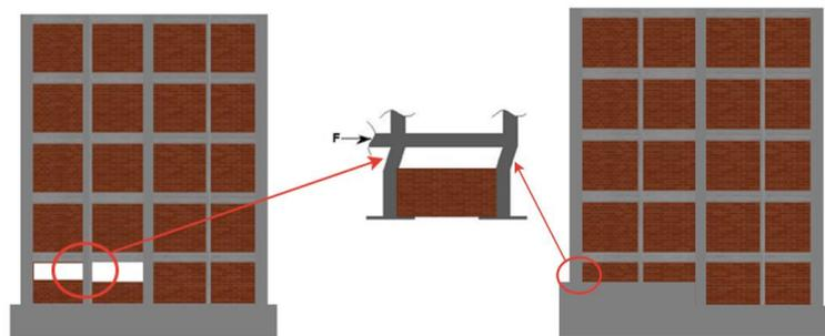
Figure 8. Short column effects in RC structures.
