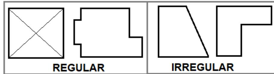
Figure 7. Determination of plan irregularities in RC structures.
