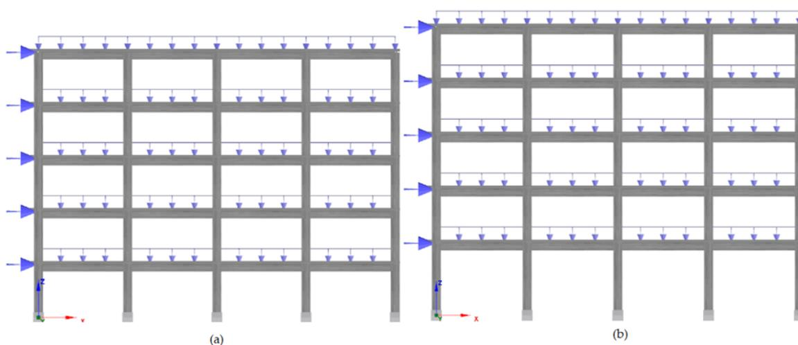
**Figure 16.** Two-dimensional models of sample RC buildings. (a) Same storey height, (b) different ground storey height.
