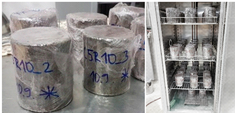
Figure 3. Samples for compressive strength and RTF determination.
