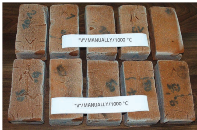
Figure 9. Appearance of manually produced brick "V" after exposure to freezing/thawing cycles
