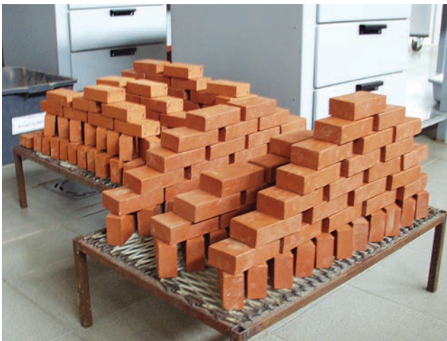
Figure 6. Bricks after firing
