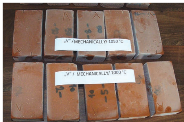
Figure 10. Appearance of mechanically produced brick "V" after exposure to freezing/thawing cycles
