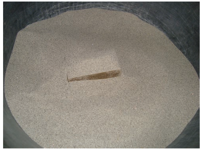
Figure 5. Covering fresh bricks with sand
