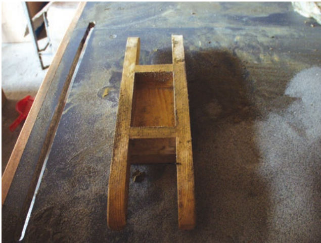
Figure 4. Mould for manual fabrication of bricks
