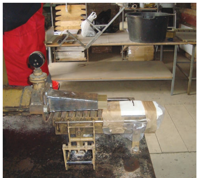
Figure 3. Mechanical fabrication of bricks
