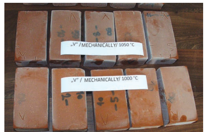
Figure 10. Appearance of mechanically produced brick "V" after exposure to freezing/thawing cycles
