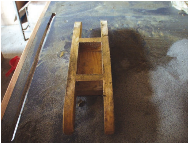
Figure 4. Mould for manual fabrication of bricks
