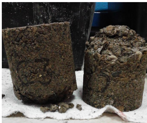
Figure 5 Specimens damaged from freeze/thaw cycling in the presence of salt
