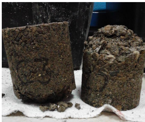
Figure 5 Specimens damaged from freeze/thaw cycling in the presence of salt
