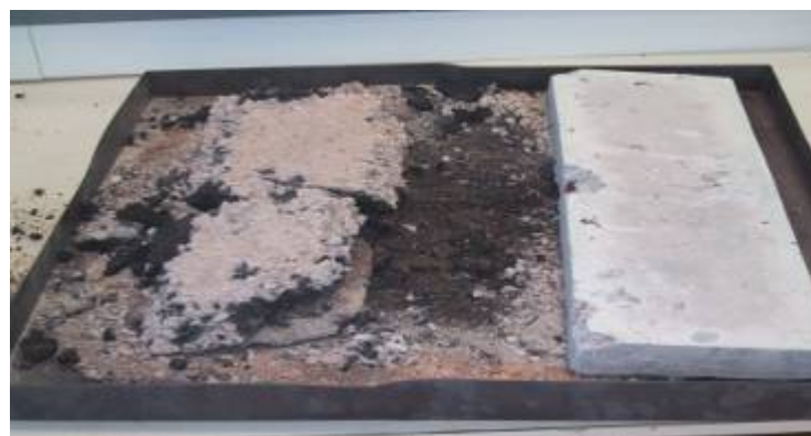
Figure 3. Comparison of asphalt (left) and concrete (right) specimens after heating to 750 °C [6]
