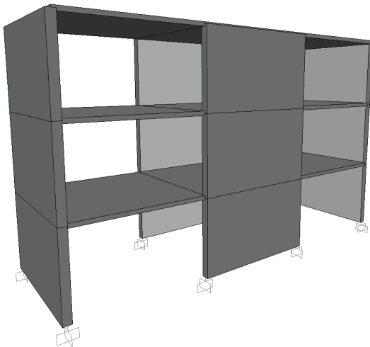
Figure 3 Structure model in SAP2000 ( n_x/n_y/n_z=1/3/3 )
