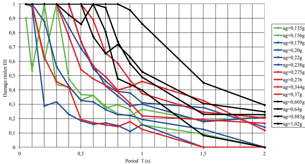
Figure 7 Spectral damage functions for RC frames defined by the following parameters:  $BS_Y = 0,1W$ ,  $K_2=0,0K_{el}$ ,  $\xi = 5\%$
