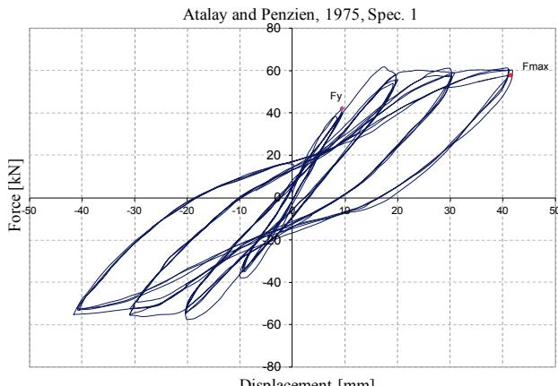
**Figure 3** RC specimen with positive post-elastic stiffness
