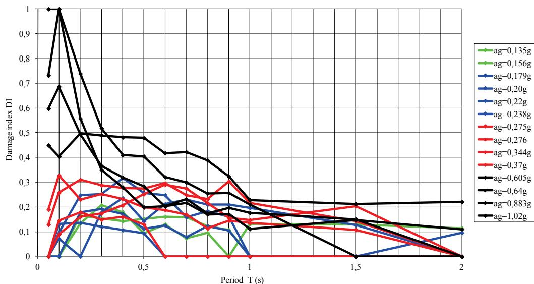
**Figure 2** Spectral damage functions for an SDOF model defined by the following parameters:  $BS_Y = 0,3W$ ,  $K_2 = 0,2K_{el}$ ,  $\xi = 2\%$
