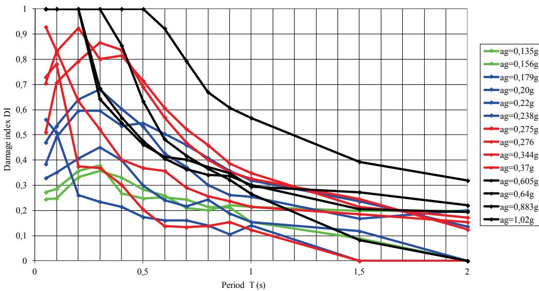
Figure 8 Spectral damage functions for RC frames defined by the following parameters:  $BS_Y = 0,1W$ ,  $K_2=0,2K_{el}$ ,  $\xi = 5\%$
