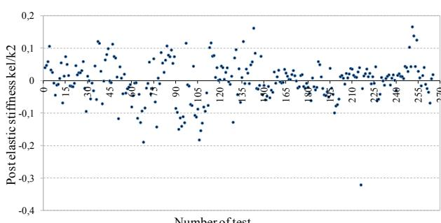
**Figure 4** Post-elastic stiffness of all RC columns specimens
