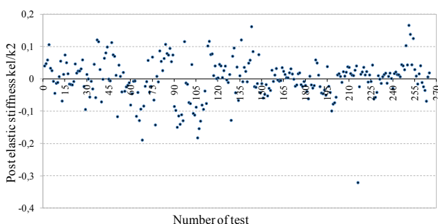
Figure 4 Post-elastic stiffness of all RC columns specimens
