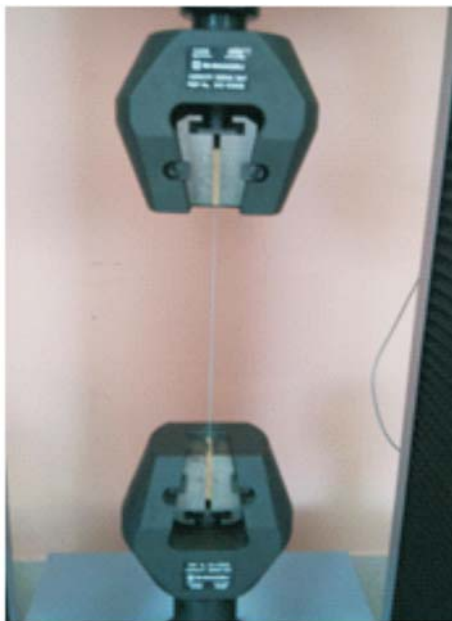
Figure 1 Testing machine and single strap sample
